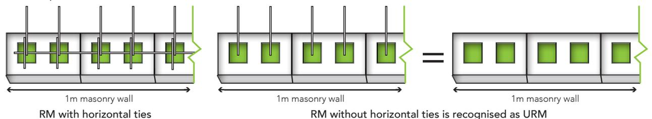
\*Please note, this picture is purely a visual representation of a 1m length of a reinforced concrete masonry wall. The spacing between each vertical reinforcement is subject to the engineers specifications, and may not necessarily be placed in each core. Please see table at the back of this spreadsheet for spacing options.
