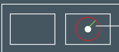
Minimum 2D, where D is the diameter of the steel reinforcing bar
