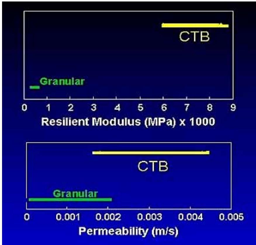
Figure 2. Permeability and Resilient Moduli for Granular and Cement Treated Base
