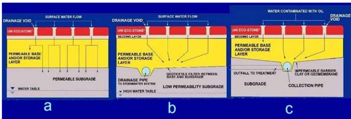
Figure 3. Recommended Cross-sections for Permeable Eco-pavements (after Rocla)
