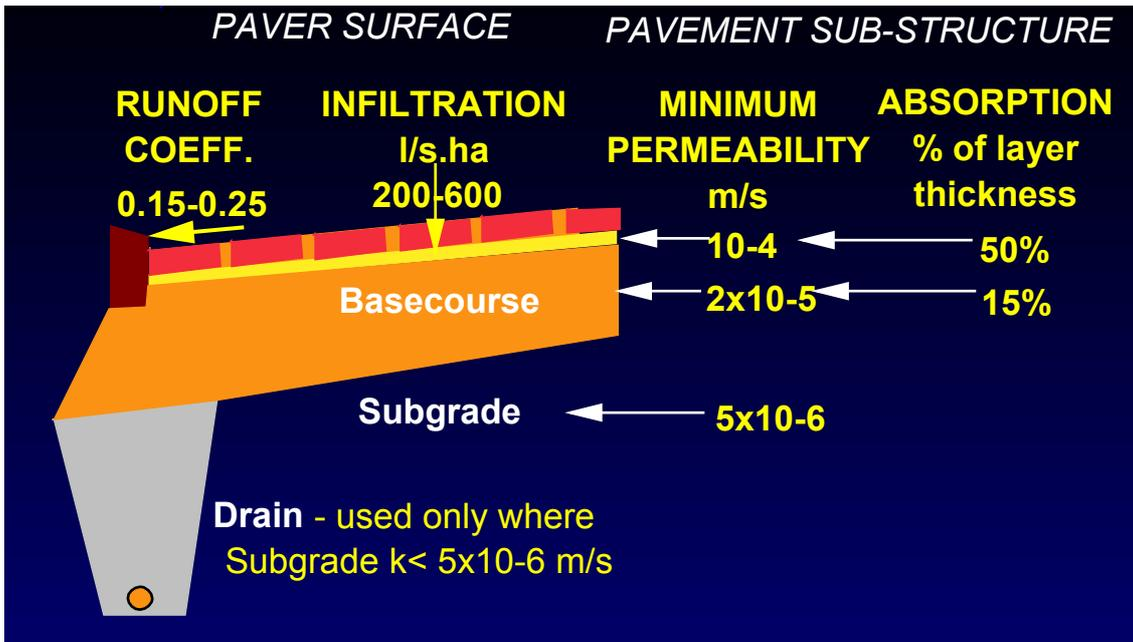
Figure 4. Typical Requirements and Design Parameters for Permeable Eco-paving
