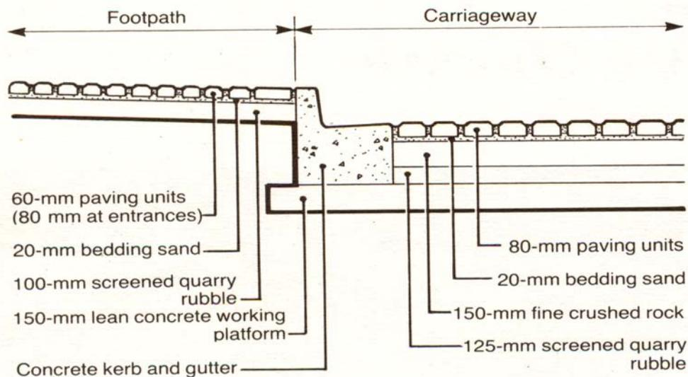
**Figure 2. Typical Pavement Cross-section**
