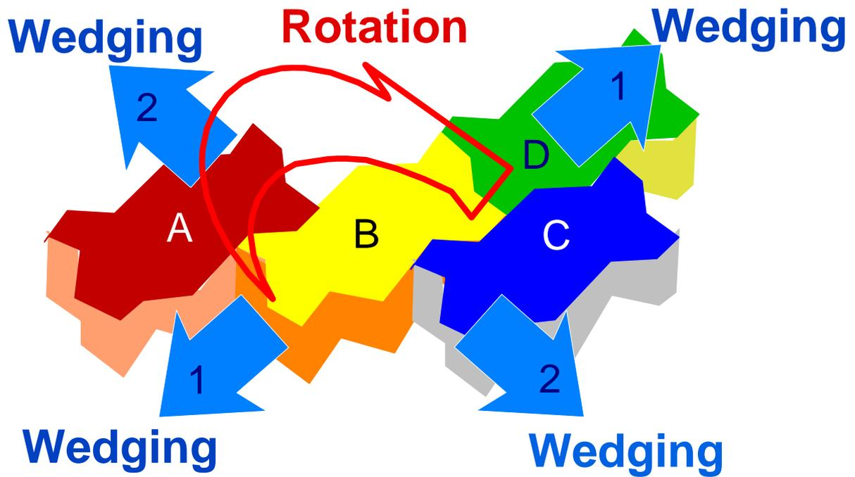
Figure 3. Effects of rotation on the wedging action of shaped pavers
