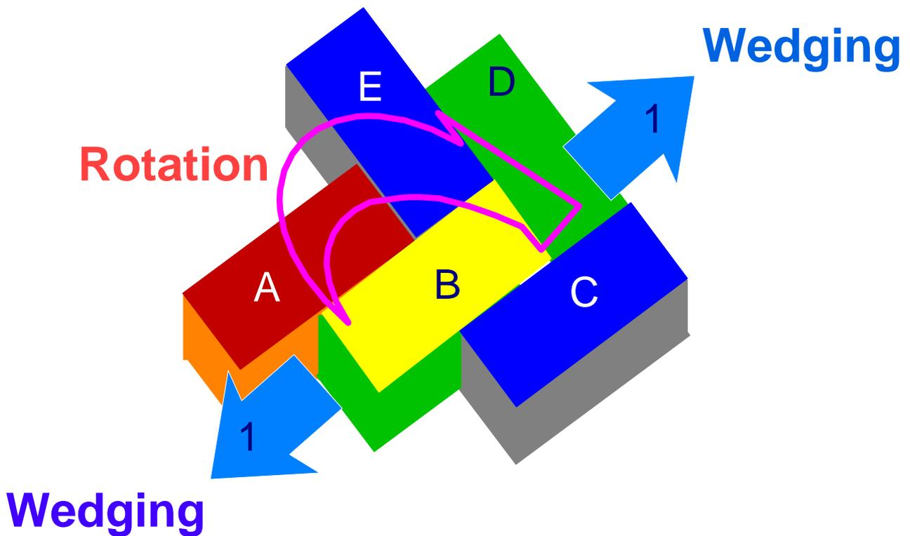
Figure 4. Effects of paver rotation on paving layed in herringbone bond.
