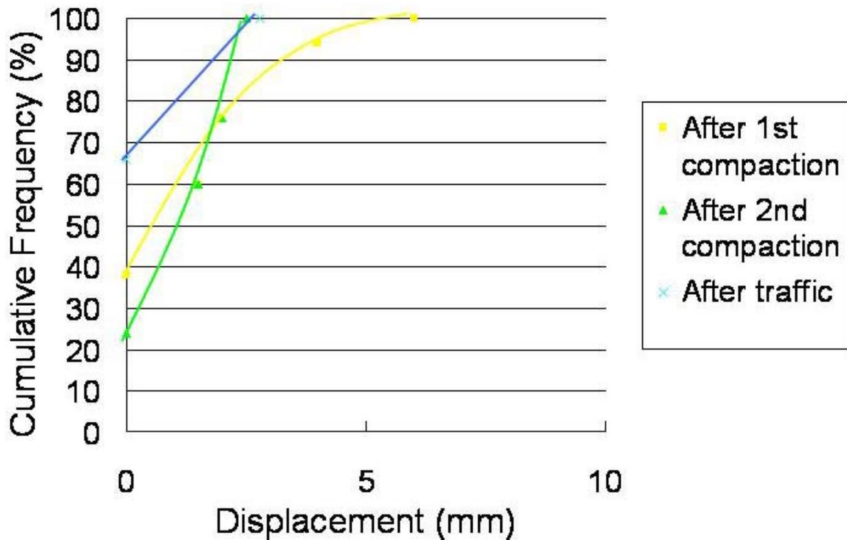
Figure 8. Distribution of displacement assuming pavers rotated about their tops
