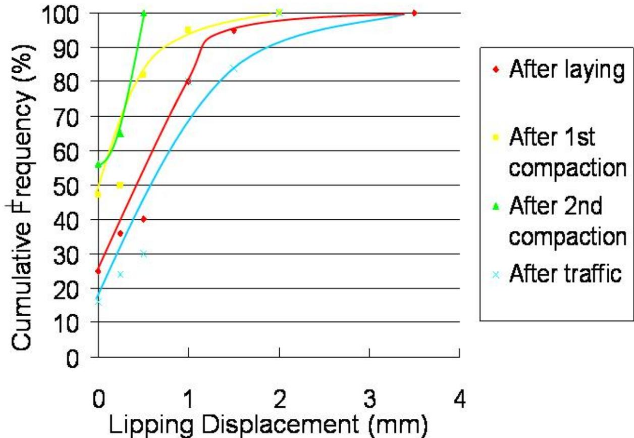
Figure 7. Lipping Displacement Measurements
