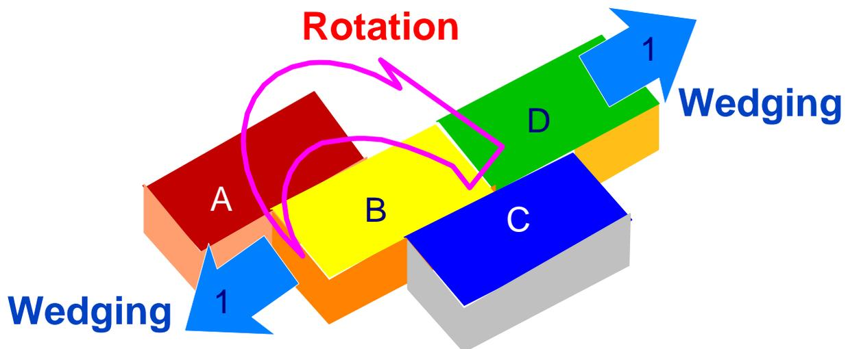
**Figure 2. Effects of rotation on the wedging action of rectangular pavers.**
