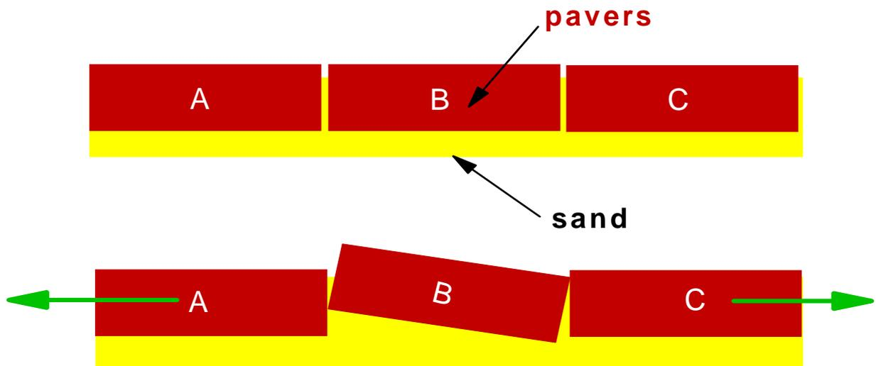
**Figure 1. Rotation of paver B causing outward wedging of pavers A and B**
