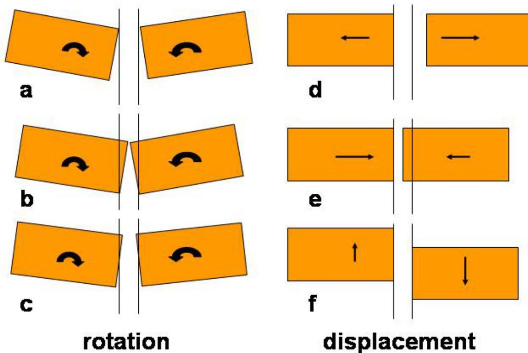
Figure 6. Movements at the Joints
