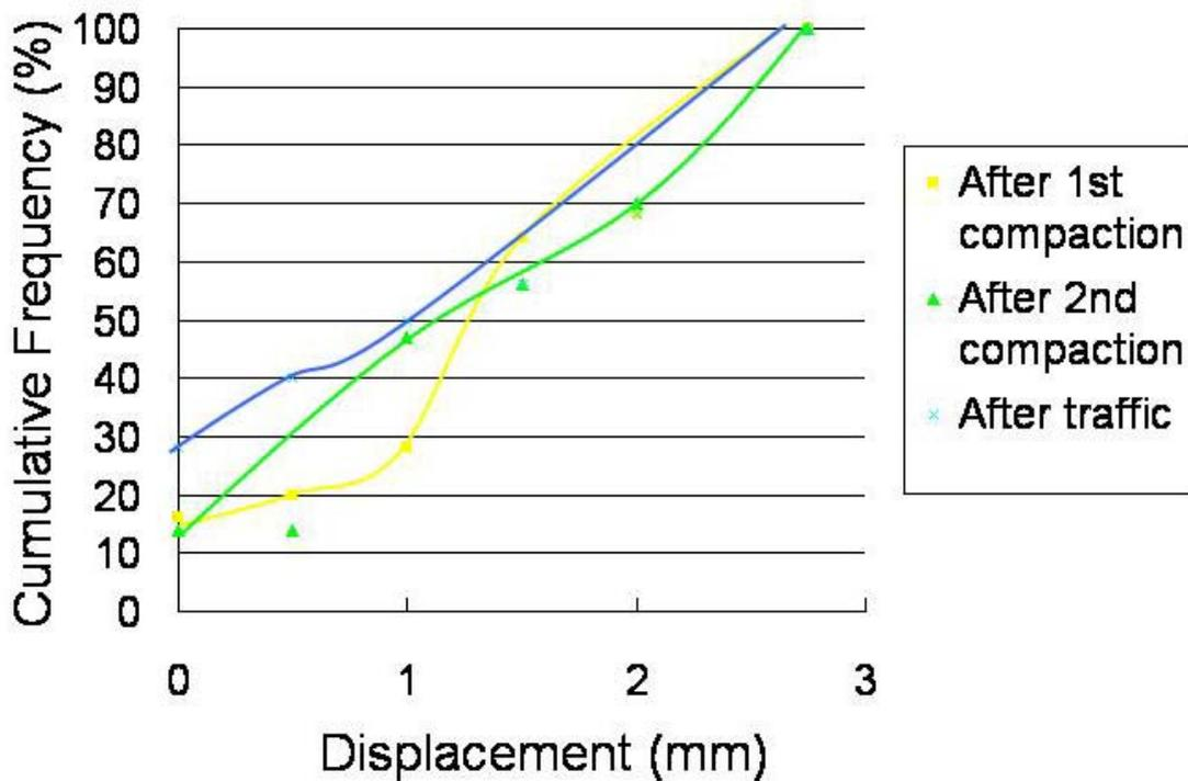
Figure 9. Distribution of displacement assuming pavers rotated about their mid points
