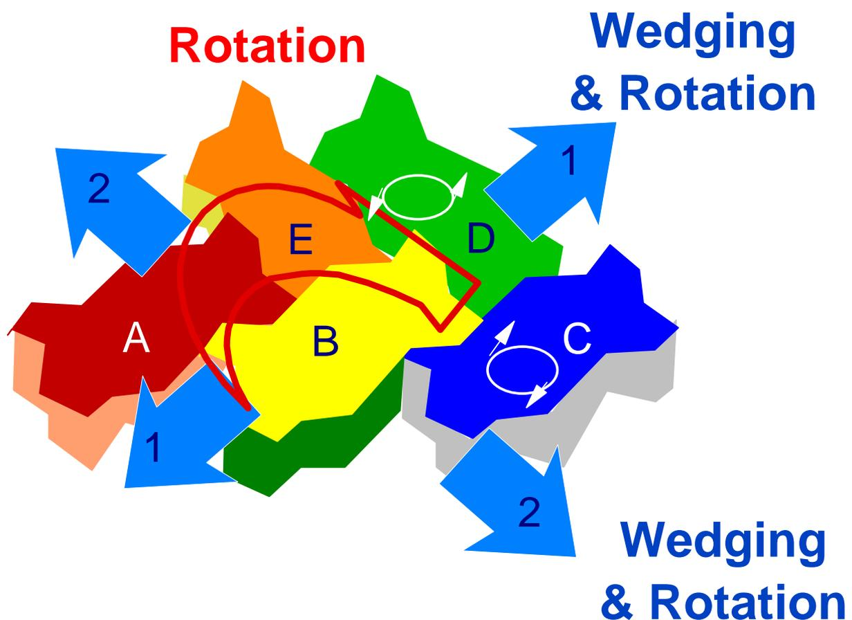
**Figure 5. Effects of paver rotation on shaped pavers layed in herringbone bond.**
