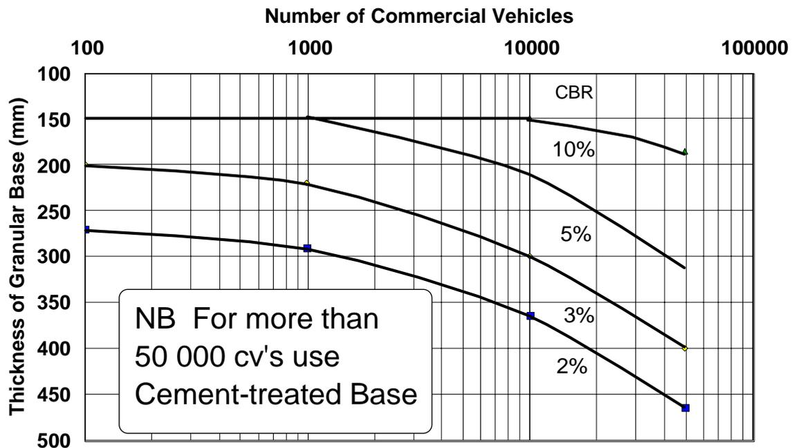
Figure 2. Granular Basecourse Thickness under Concrete Flags Carrying Less than 50000 Commercial Vehicles
