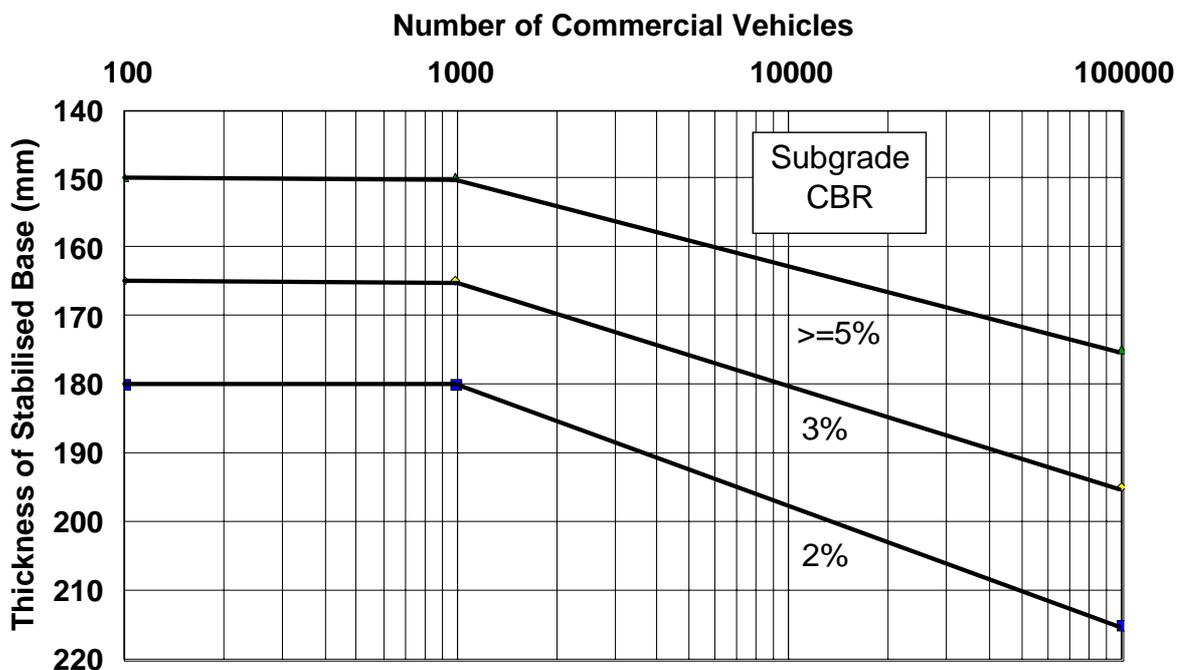
Figure 3. Cement Stabilised Base Thickness under Concrete Flag Pavements Carrying more than 50000 Commercial Vehicles
