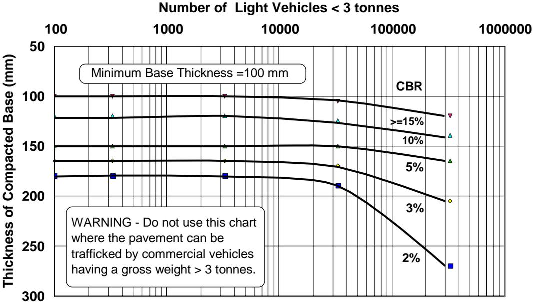
*Figure 1. Basecourse Thickness under Concrete Flags subject to Light Vehicles only.*
