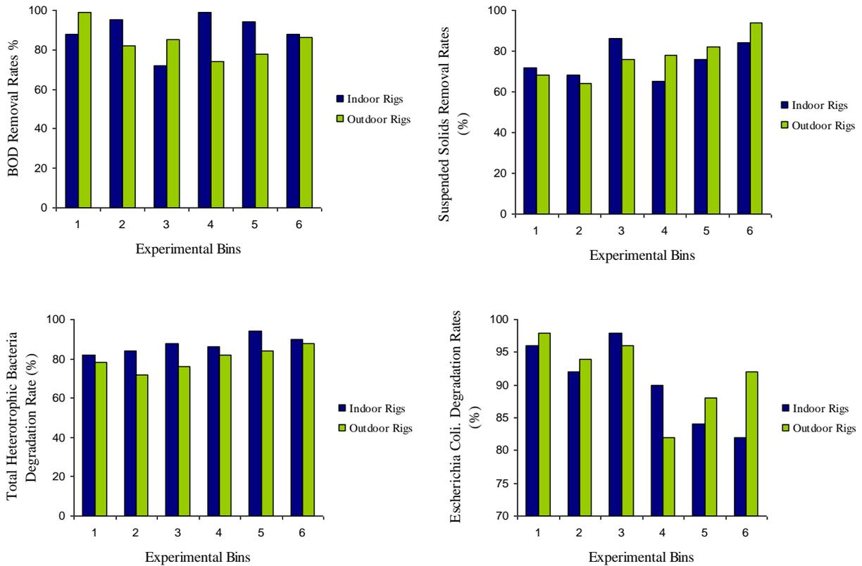
**Figure 3. Mean Removal rates for BOD5, Suspended Solids, Total Heterotrophic Bacteria and E.Coli from June 2006 to March 2009.**
