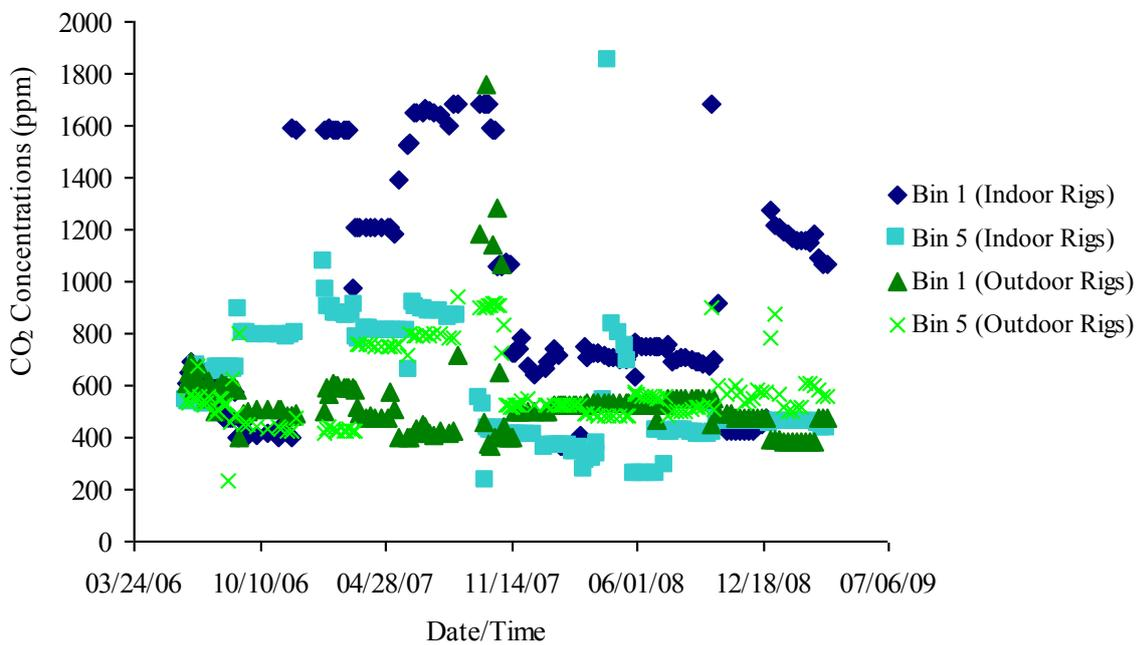
**Figure 3. Average CO2 (ppm) measured for Bins 1 and 5, indoor and outdoor bins respectively, from June 2006 to March 2009.**
