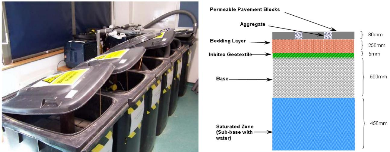
Figure 2. Indoor Experimental rigs and schematic layout of permeable (pervious) pavement systems with integrated ground-source heating and cooling elements.
