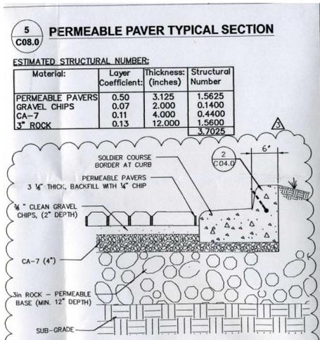
Figure 2. Permeable paver typical section.
