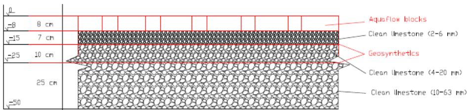
Figure 0. Components of a pervious pavement in Santander, Spain.
