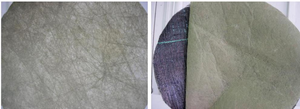
Figure 2. Geotextile materials: a) Infiltration and b) One Way.
