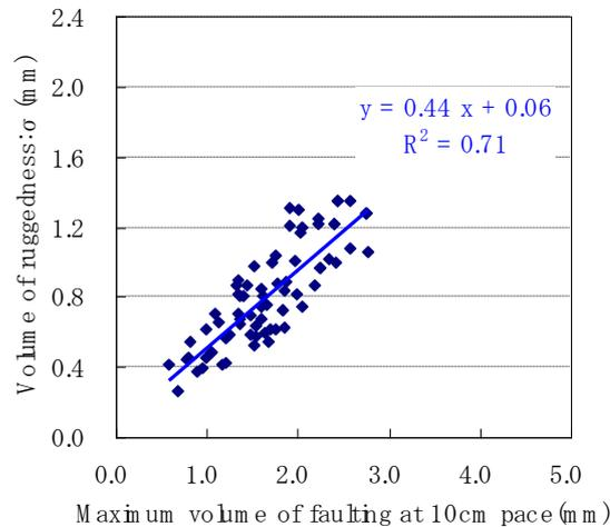
Figure 4. Relations between Maximum Volume of Faulting and Volume of Ruggedness.
