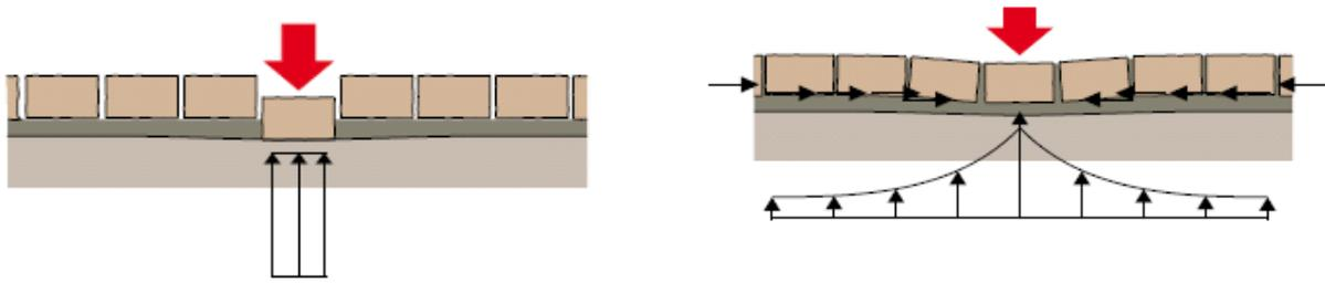
Figure 4. Structural behavior of a CBP with (left) and without joint sand (right).
