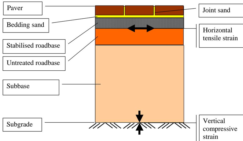
**Figure 3. Swedish CBP system containing a stabilized road base. Horizontal tensile strain in the stabilized road base, if any and vertical compressive strain are the design criteria used.**
