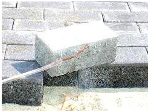
**Figure 1. IL block specimen installed with Type-T thermocouple.**
