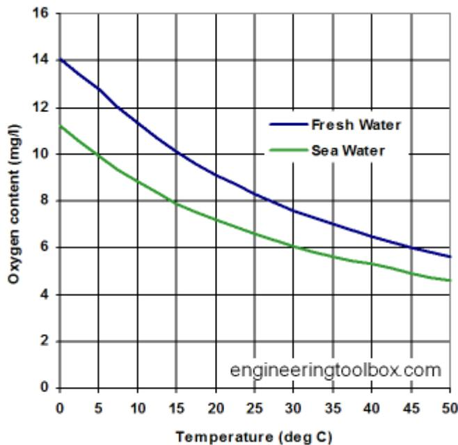
**Figure 2. Relationship between Temperature and Oxygen Content.**
