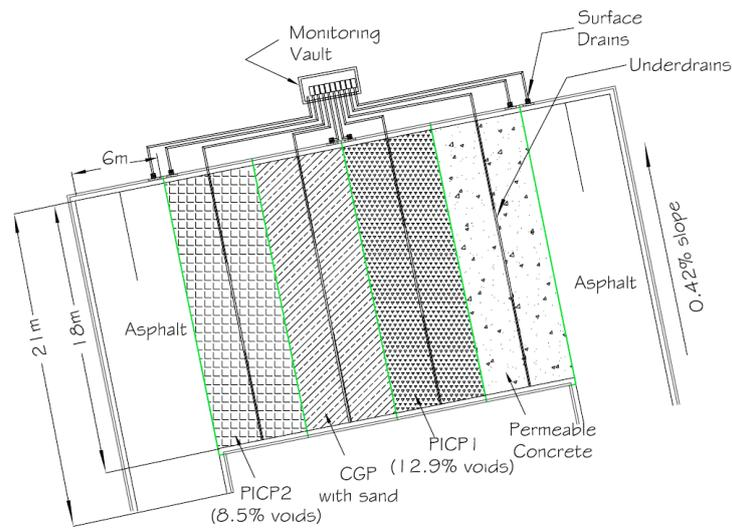
**Figure 2. Permeable pavement parking lot design (plan view).**
