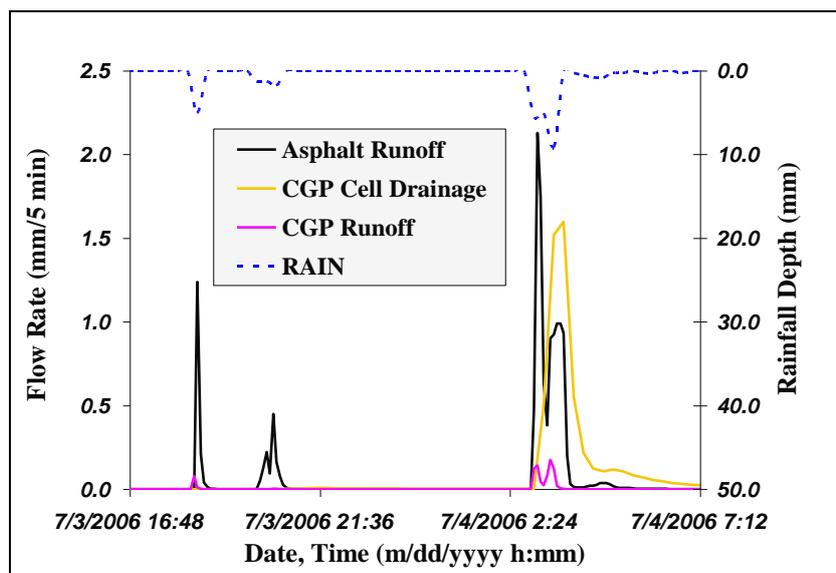
**Figure 3. Asphalt runoff and CGP runoff and drainage for 32.8 mm event on 7/3/2006.**
