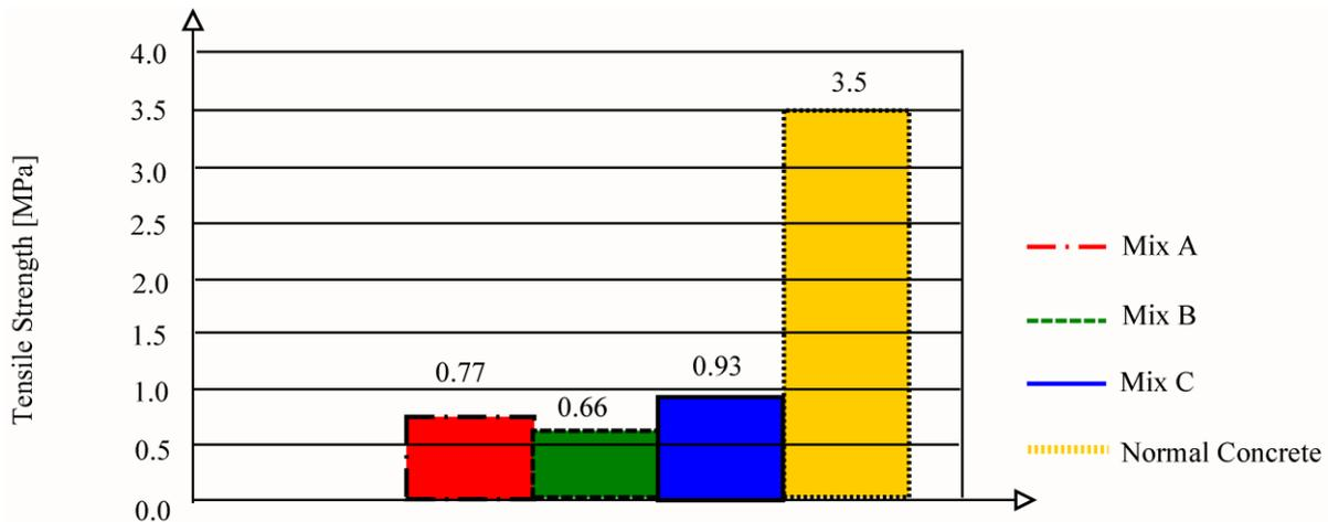
Figure 5. Indirect Tensile Strength Test Results.
