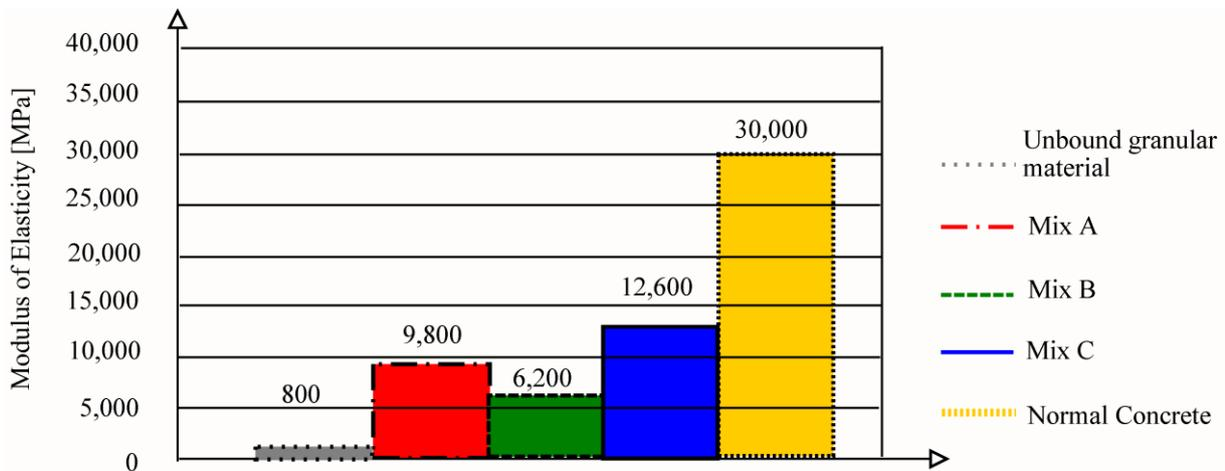
Figure 6. Test Results – Static Modulus of Elasticity.
