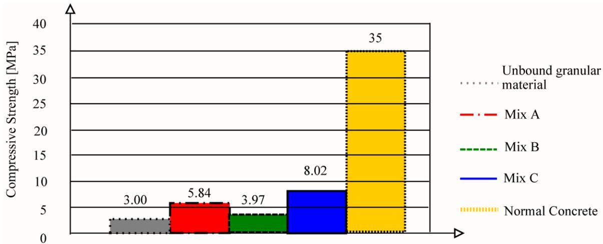
Figure 4. Unconfined Compressive Strength Results.
