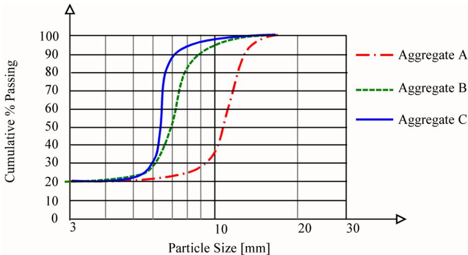
Figure 1. Grading curves.
