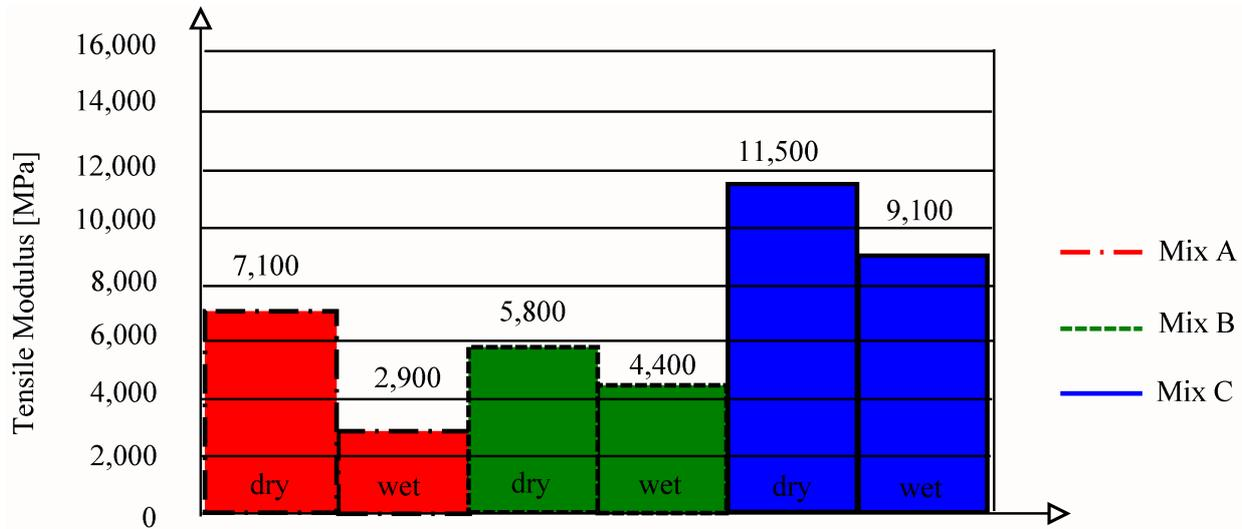
Figure 7. Test Results – Modulus from Repeated Indirect Tension Tests.
