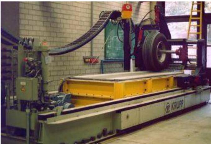
**Figure 3. Photo of the Street Testing Machine of Ruhr University Bochum.**
