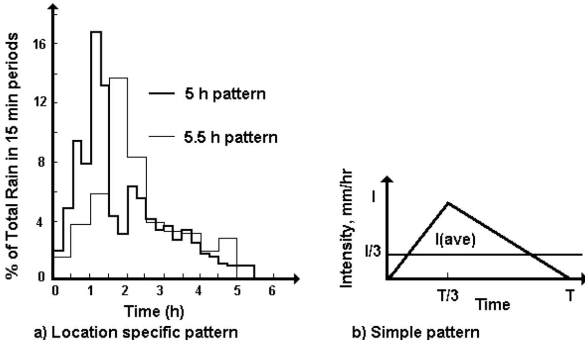
Figure 3. Storm temporal patterns applied to design average storm intensity.
