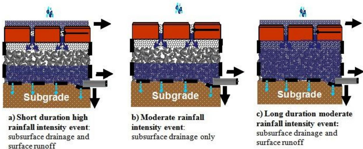
Figure 4. Flood storage and combined maximum discharge analysis modes.
