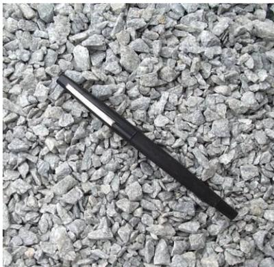
**Figure 5. ASTM No. 8 stone for bedding and joints.**
