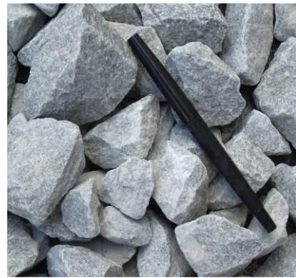
**Figure 7. ASTM No. 2 stone for the subbase.**
