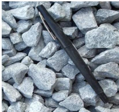
**Figure 6. ASTM No. 57 stone for the base.**
